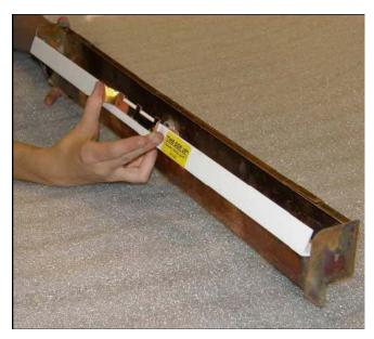
Now you will need to adjust the lower tabs to shift the water to the areas that are dry. These tabs act like dams controlling where the water will flow. If the center is not getting enough water, pull the tabs down so they hold more water in the center. Or, to allow more water to one side or the other you can flatten one or both a little to shift water to either side. You may need to adjust the tabs a few times to get the water to flow properly.
