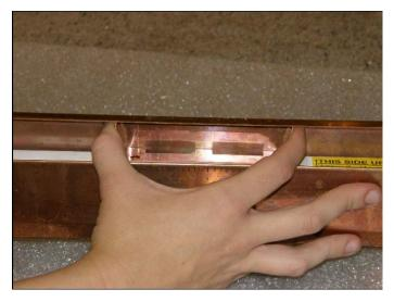
When replacing it; once it is in, be sure it is square to the Water Distribution Unit, then bend the upper tabs up until they push against the top lip of the Water Distribution Unit. Doing this will keep the Baffle firmly in place and allow the water to flow properly.
