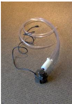
Pump with manifold and hoses attached - outside the stand
