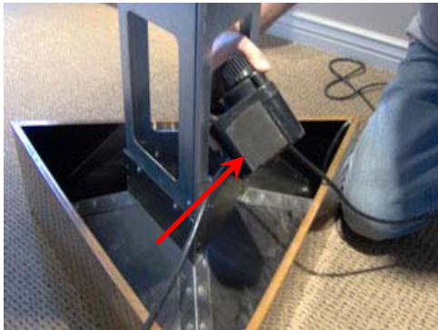
Inserting Pump with pump pad attached
